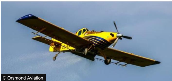
An electronic system for fire operations allows a full-salvo dump to be programmed - either the full load in two seconds, a lengthened release or multiple partial releases. There is an infrared system available which can enhance forward visibility in poor conditions such as smoke. "It's a simple little ag airplane but the technology is really cool...Everyone is investing more and more in using new technologies to do a better job," Rojek adds. *To be continued next issue.*
